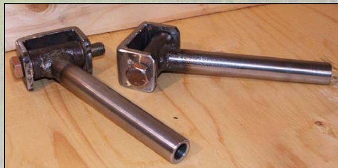
The 20mm axle hubs sat on a pair of custom machined hollow tubes that were welded at an angle to another tube that carried a pair of brass bushings.
