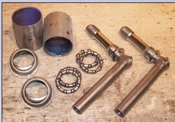
The steering parts to carry 20mm axle hubs
