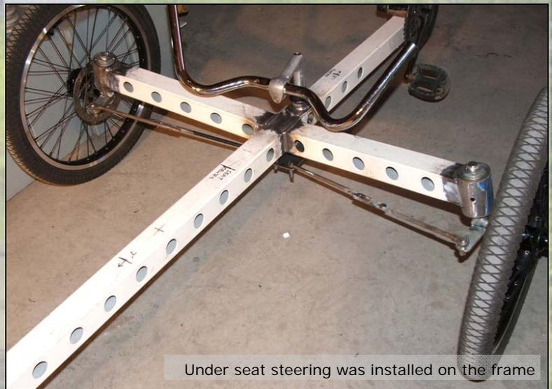
Under seat steering was installed on the frame
