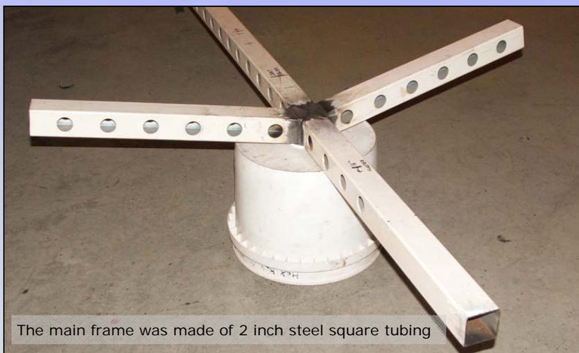
The main frame was made of 2 inch steel square tubing
