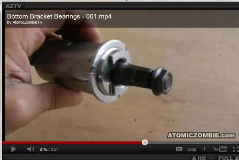
The crank axle is a hardened steel rod that includes a pair of machined bearing races, tapered square ends, and either a bolt or internally threaded section at each end to affix the crank arms.
